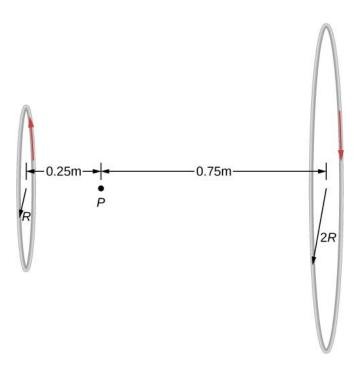
5.2 The magnetic flux through the loop shown in the figure increases according to the relation  $\phi_B = 6t^2 + 7t$  where  $\phi_B$  is in milliwebers and t is in seconds.
