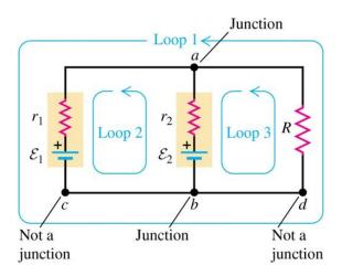
3.5 Consider a circuit below and calculate currents,  $I_1$ ,  $I_2$  and  $I_3$ .
