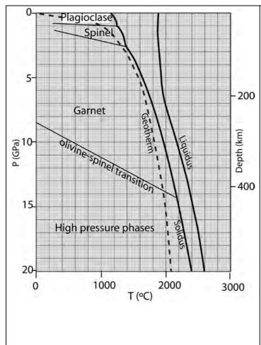
The diagram to the left shows the solidus and liquidus for the mantle, the geotherm, and the stability fields for selected minerals.
