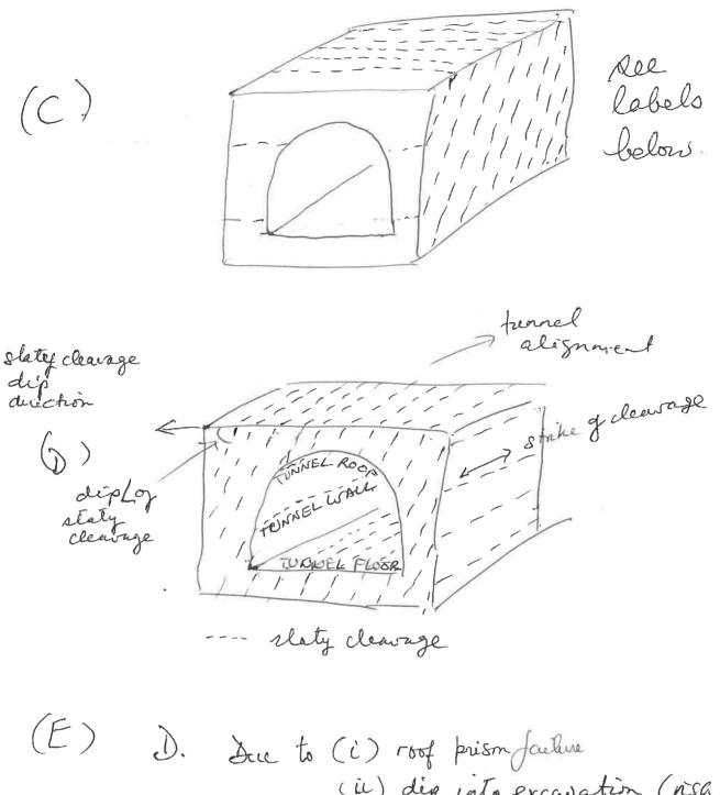
(E) D. Due to (i) roof prism facture
