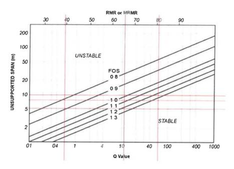
(D) In the figure below, select the correct plot lines and read off the stand-up time for a tunnel with a span of 5m. Read the time on the top horizontal axis. (2 marks)
