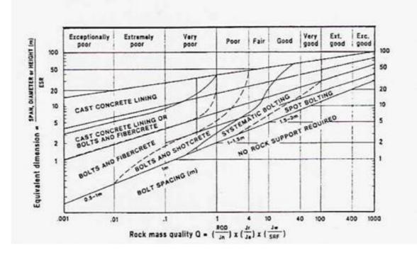
(G) What is the preventative work necessary for the excavation to be stable. Use the diagram above. (2 marks)
