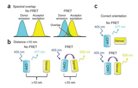
(i) The figure labelled **a**, **b** & **c** is a FRET diagram, which is explored by molecules during spectroscopic experimental measurements. Give a detailed description of how this mechanism is used to effect excitation and de-excitation [10 Marks]
