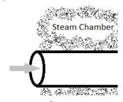
0.01 kgs<sup>-1</sup> of a pharmaceutical liquid, consisting mainly of water (assume same physical properties), is to be sterilized by heating from 300 K to 350 K in a straight 0.02 m internal diameter stainless-steel tube. For this tube, a uniform surface temperature of 373 K is maintained by steam condensing on the outer surface of the tube. Thermal resistance of the tube wall may be neglected, and fully developed velocity and temperature profiles may be
