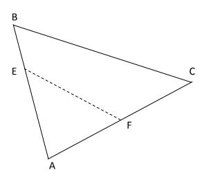
It is required to divide the triangular area ABC into 2 equal areas by a straight line drawn from the given point E on the side AB to a point on F on the side AC.
