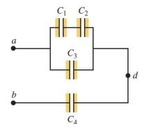
Calculate the equivalent capacitance  $C_{ab}$  between points *a* and *b*. (5)
