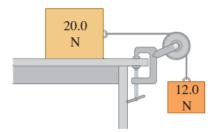
Traveling at constant speed, the 20.0 N block moves 75.0 cm to the right and the 12.0 N block moves 75.0 cm downward.
