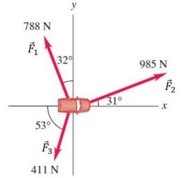
Determine the magnitude and direction of the resultant force on the car. (7)
