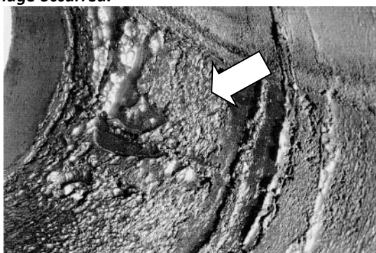
Figure 2.5—Photographs showing areas to the (a) right and (b) left of the top relatively undamaged surface. The arrow in (a) indicated where the leak occurred.
