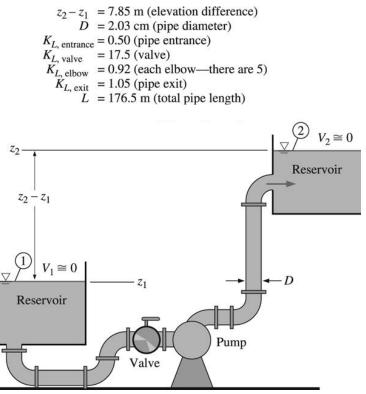
The expression in the pump's performance curve contains the shutoff head  $H_0 = 24.4$  m of water column and the coefficient a = 0.0678 m/Lpm<sup>2</sup>. Estimate the capacity delivered by the pump if the coefficient of pipe friction is 0.1024. (8)
