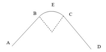
AB and CD are two roads straights that must be linked by a circular curve BEC.
