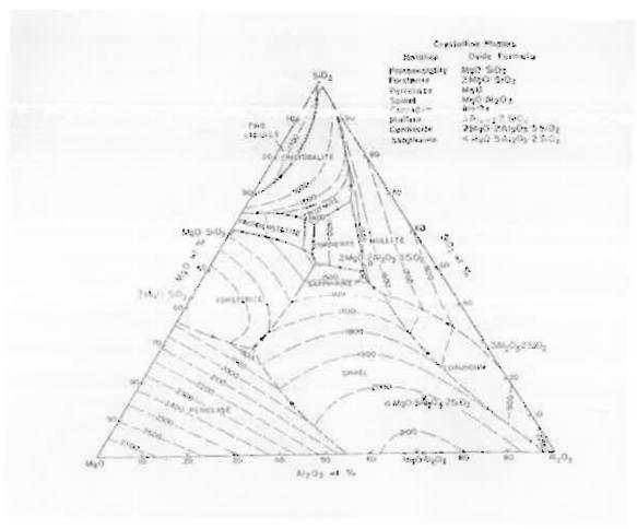
Figure 1. Phase diagram of SiO2-MgO-Al2O3
