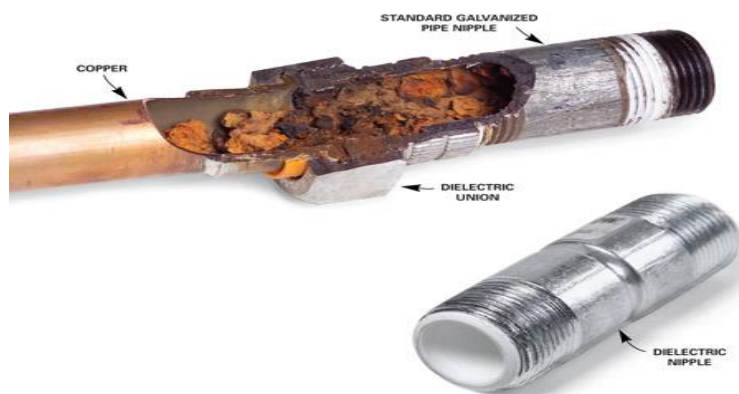
Figure 1: Corrosion of two pipes
