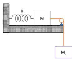
a) When the spring is stretched 0.2 m, the system is at rest. Calculate the mass of  $M_L$ . [6]
