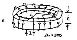
A toroid of square cross section is wound with N = 200 turns, as shown in the figure. The inner and outer radii of the toroid are a = 20 cm and b = 25 cm, respectivally. Its height is h = 5 cm. The relative permeability of the magnetic material is  $\mu_r = 500$ .
