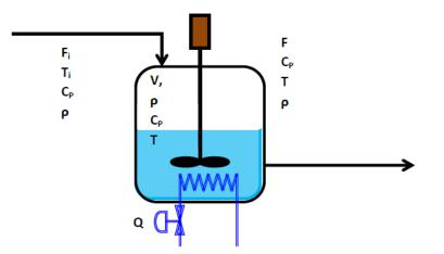
The heat, Q is changed by manipulating the flow of saturated steam,  $F_S$  (mass/time). The heat added to the liquid process stream can be calculated from the heat of condensation of steam as  $Q = \lambda_S \cdot F_S$ .
