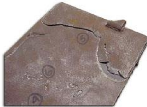
Figure 1 Casting defect in steel cast component
