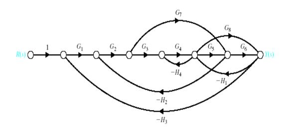
Formulate the transfer function of the diagram above, using Mason's Rule.
