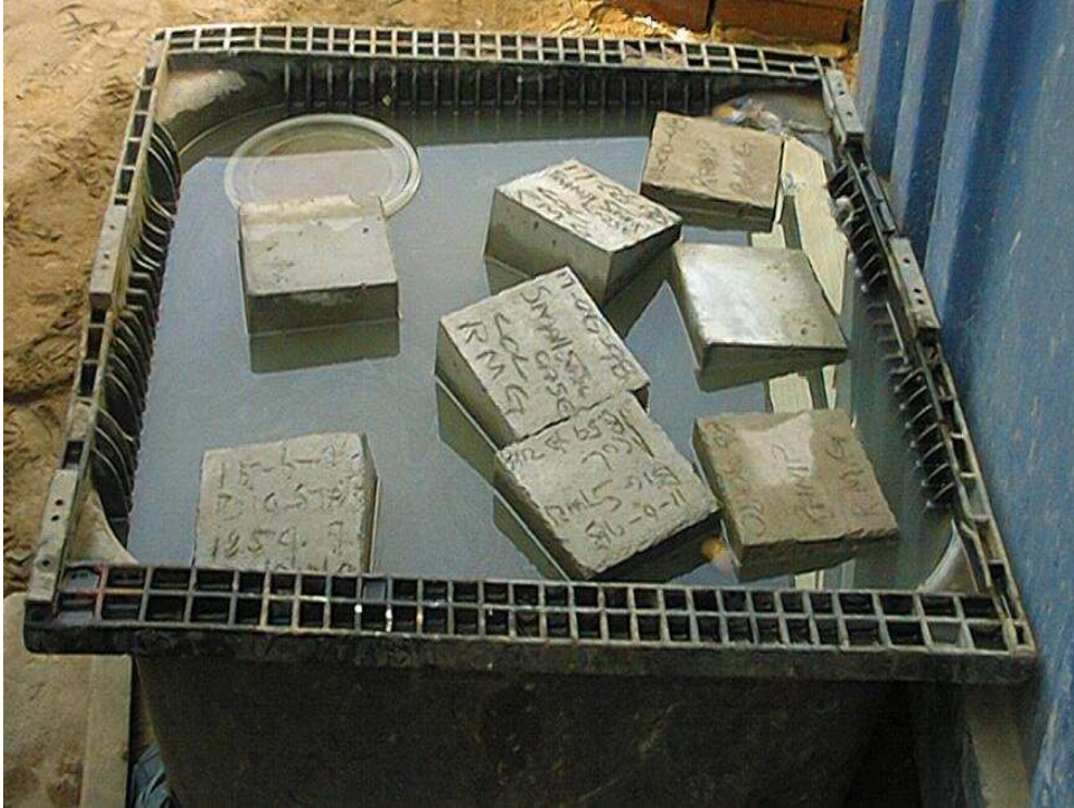
Picture 1: Concrete cubes being cured on site
