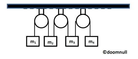
Given that  $m_1 > m_2 > m_3 > m_4$  in the pulley system, with the aid of detailed free-body diagrams and equations, derive the acceleration *a* of the system in terms of  $m_1$ ,  $m_2$ ,  $m_3$ ,  $m_4$  and g only. (4)
