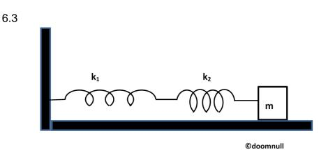
At equilibrium position neither of the springs with stiffness constants  $k_1$  and  $k_2$  respectively is stretched or compressed. The mass *m* is displaced *x* from equilibrium and then released from rest. Derive the expression
