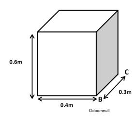
A uniform rectangular block of density 850 kg/m<sup>3</sup> rests on a horizontal table. Calculate:
