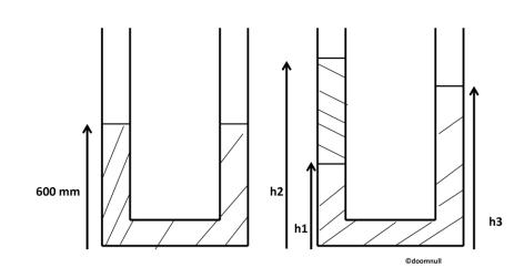
A U- tube of internal cross-sectional area 10 mm<sup>2</sup> contains water as shown in the diagram. A volume of  $10^3$  mm<sup>3</sup> of oil of density 800 kg/ m<sup>3</sup> is introduced into the left arm of U-tube. No mixing takes place and the system comes to equilibrium. Calculate the height of the three interfaces,  $h_1$ , $h_2$  and  $h_3$ .
