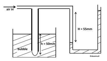
The sketch shows an apparatus for measuring surface tension. When air is blown into the apparatus, bubbles are emitted from the end of the tube, which
