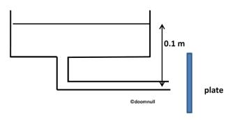
Water flows out of a tank through a tube 5 mm in internal diameter and is discharged horizontally, striking a vertical plate. The outlet is 0.1 m below the free surface of the water, and the cross-sectional area of the tank is extremely large compared with that of the tube. Calculate:
