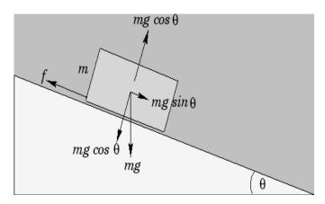
Prove that the coefficient of kinetic friction is  $\mu_k = \tan \theta$  (05)
