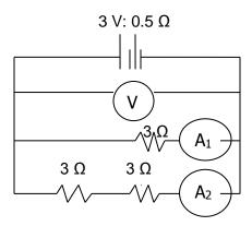
5.1.1. The reading on the voltmeter.
