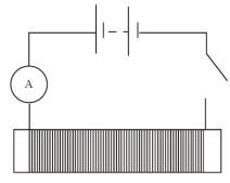
When the switch is closed, the ammeter reading gradually increases from zero to a maximum value. What is the explanation for this gradual growth of current?
