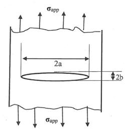
Inglis found that for an elliptical internal hole subjected to an applied stress  $\sigma_{app}$  was magnified at the ends of the major axis of the ellipse so that
