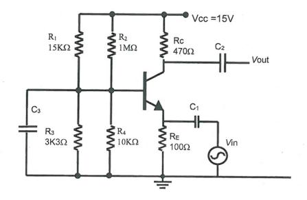
2.1. Draw and label a complete circuit of the h-parameter small signal model of the eireuit above. All four h-parameters must be clearly indicated. (10)
