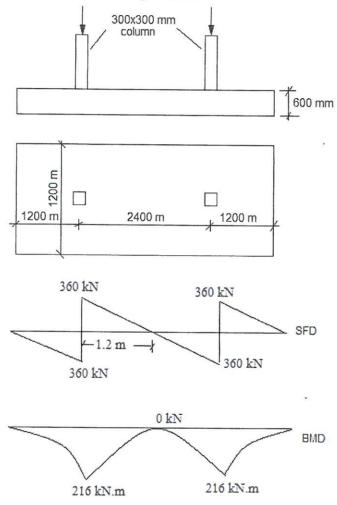
(i) Design the longitudinal (tension) reinforcement
