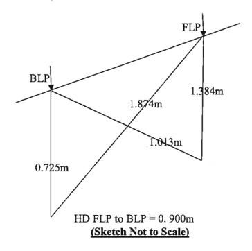
Two line pegs BLP and FLP were established in an orepass and the measurements were taken as shown in the sketch below.
