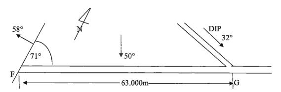
The figure above represents a reef drive which has intersected a fault at point F. A raise is developed from point G, 63.000 metres north-east of F at a dip of 32°, in a westerly direction.
