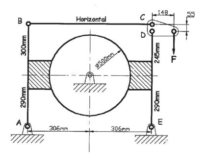
Calculate the force F that has to be applied at the (CDF) in order to obtain a braking torque of 1755 Nm for a clockwise rotating drum. Each block is rigidly fixed to the lever and the coefficient of friction is 0.32 at the brake drum.
