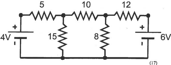
2.2 By conducting a Star to Delta transformation on Star ABC calculate the total current.
