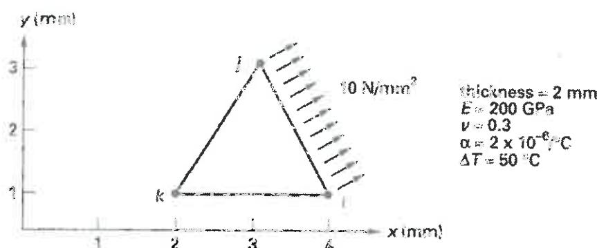
**Figure 4 2D Plane stress element (dimensions in mm)**
