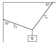
1.2 A car engine of weight 2000 N is lifted by means of a chain and pulley system. The engine is initially suspended by the chain, hanging stationary. Then, the engine is pulled sideways by a mechanic using a rope. The
