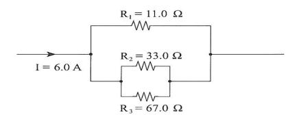
6.2 Determine the value of resistor R in the circuit shown below. (3)
