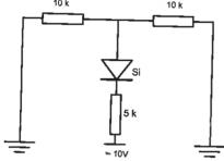
Calculate the volt drop across the 5 k resistor.
