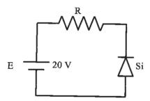
When a voltmeter is placed across the diode, it will read a voltage approximately equal to:
