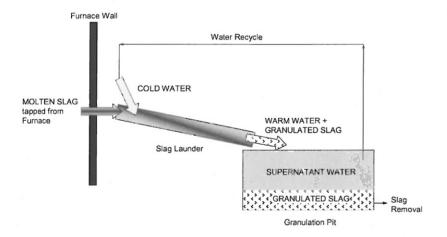
Hint: Granulation means that the slag freezes upon contact with the cold water and becomes a solid, consisting of small particles. The heat that is transferred to the cold water when the slag is cooled is of course the same that it would take to heat up and melt solid slag. Use the mean heat capacities for both slag and water, but do not forget to take the heat of fusion for slag into account; this is given in the table under Ho298 for Fe2SiO4liq.
