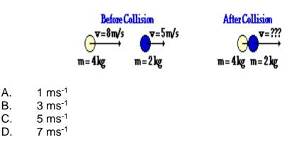
19. Determine the unknown velocity value in the system shown below. Assume that the collisions occur in an isolated system.
