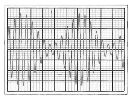
The waveform above is displayed on an oscilloscope that is set to 2 V per division and 0.02 ms per division. Consider this, to determine:
