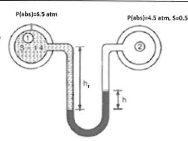
between the mercury levels in the two limbs). The density of mercury is 13600 kg/m<sup>3</sup> and the density of water is  $1000 \text{ kg/m}^3$ . Take  $g = 9.81 \text{ m/s}^2$ .
