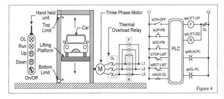
Design and sketch a PLC ladder program for the operator to control the lift via the hand held unit. Use the symbolic input and output connection names shown in the table below, in your PLC program. Only N/O or N/C contacts, output and internal relays may be used.
